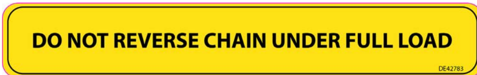
Item - D Part No: DE42782 - Reversing apron chain while spreader is fully loaded will cause front apron shaft breakage.
