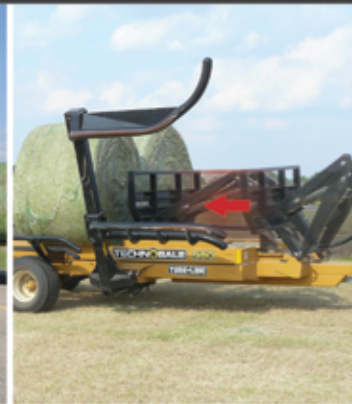
Scissor style pusher reduces cycle time.
