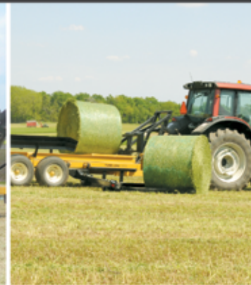
Pickup arm gently spins bale into position.
