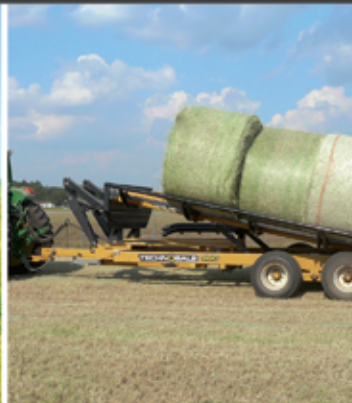
Hydraulic Cylinders raise the bed up to 45 degrees to gently unload bales.
