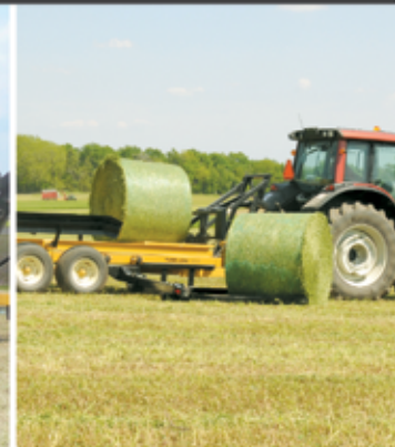
Pickup arm gently spins bale into position.
