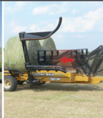
Scissor style pusher reduces cycle time.
