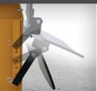
The variable position chute allows you to go from bedding, to feeding, to windrowing.
