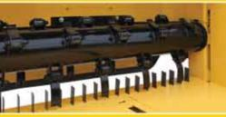
The adjustable cutting knives can be raise to further process material cutting it as small as 4.5 inches for more uniform bedding material.
