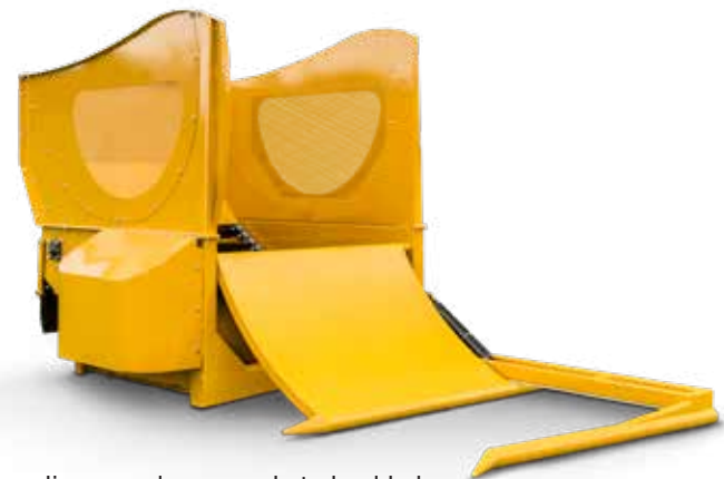
Loading arm down, ready to load bale.
